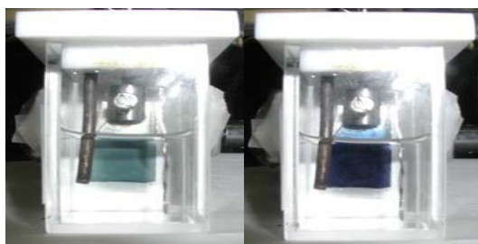
"Oxidation (light blue) and reduction state (blue) of a electrochromic polymer"
